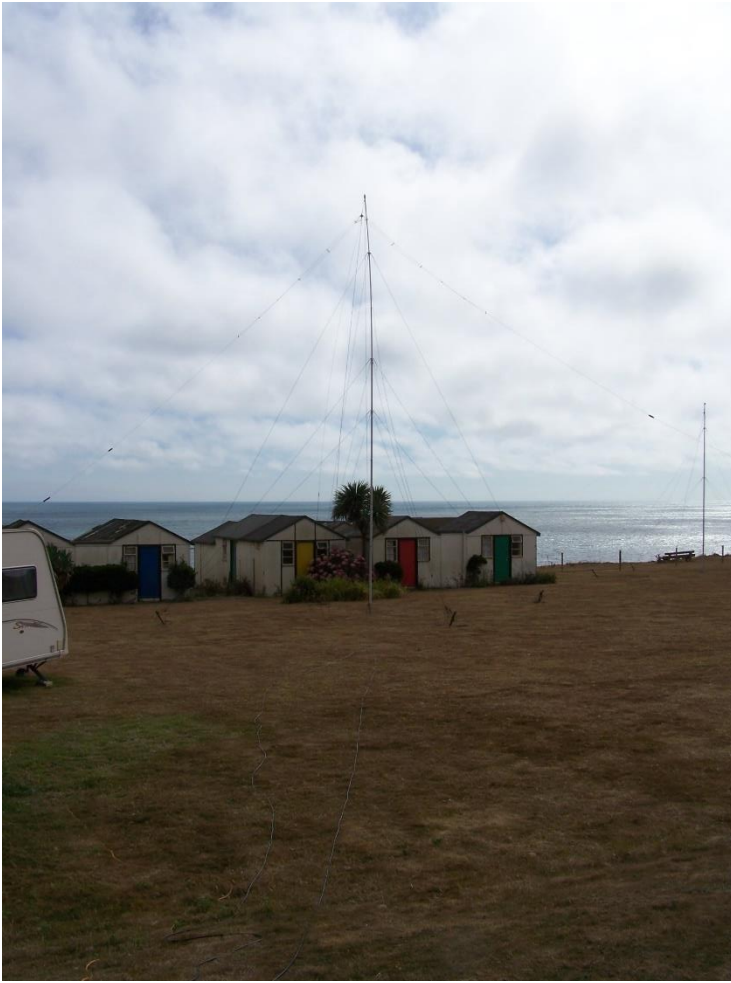
ANTENNAS AT G4ALE/P Centre – FAN DIPOLE FOR 80/20/10m, Right – 40m DIPOLE FOR 40/15m
