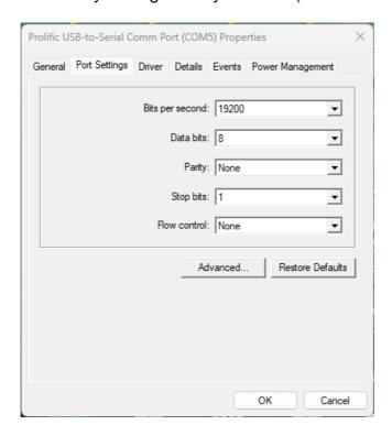
I also had to reset my COM port to match the software I was using for the rig (WSJT-X) and this can be changed under the Advanced.. button:
