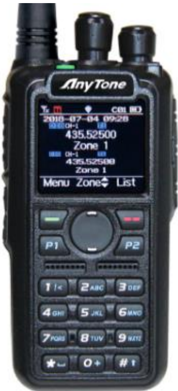
Anytone AT-D878UVII Plus Dual Band 2m/70cm, dual mode 5W transceiver
