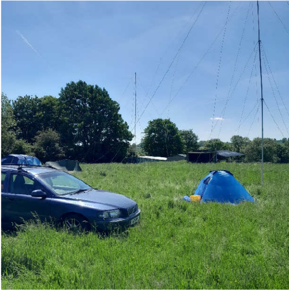
2 x 45ft MASTS SUPPORTING 160m DOUBLET ANTENNA
