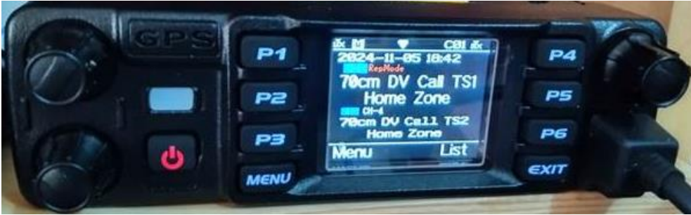
Anyone AT-D578UVIII transceiver used as repeater in DMR demonstration.
