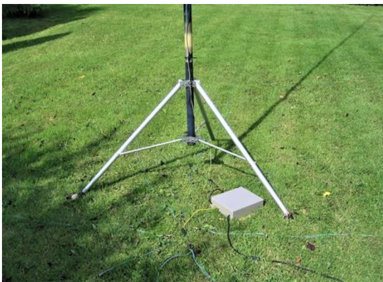
ANTENNA TRIPOD AND ATU
